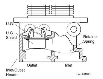
To test the operation of the Unitherm Governor, place in hot water (over 110°F) and watch for movement against spring. If there is no movement, replace unit.
